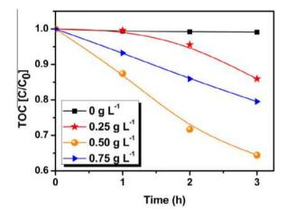
Fig. 5. Effect of catalyst dosage [Experimental conditions: LaFeO<sub>3</sub> and 4-chlorophenol (1.25  $\times$  10<sup>-4</sup> M) were ultrasonicated (40 kHz) for 3 h].
