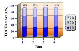
Fig. 10. Recyclability test [Experimental conditions: LaFeO<sub>3</sub> ( $0.5 \text{ g L}^{-1}$ ), 4-chlorophenol ( $1.25 \times 10^{-4} \text{ M}$ ) and KPS (0.5 mmol) were ultrasonicated (40 kHz) for 3 h].
