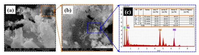
Fig. 2. (a and b) SEM images and (c) the corresponding EDS spectrum of LaFeO3 catalyst [inset: wt% table].
