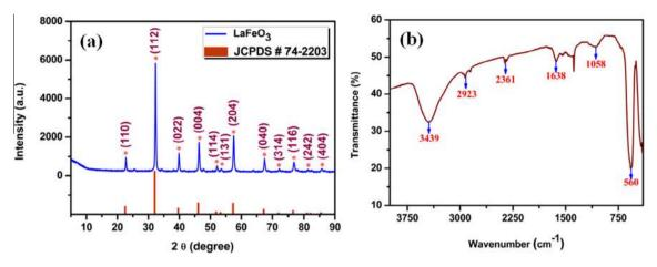
Fig. 1. (a) Powder XRD pattern and (b) FT-IR spectrum of LaFeO<sub>3</sub> catalyst.
