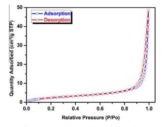
Fig. 4. N<sub>2</sub>-adsorption/desorption isotherm of LaFeO<sub>3</sub> catalyst.
