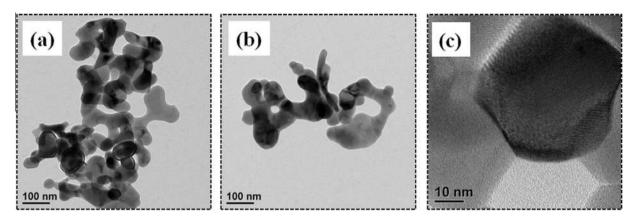
Fig. 3. TEM images of LaFeO<sub>3</sub> catalyst with different magnification (a and b) 100 nm and (c) 10 nm bar scales.
