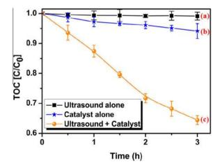
**Fig. 7.** TOC as a function of time [Experimental conditions: (a) 4-chlorophenol  $(1.25 \times 10^{-4} \text{ M})$  were ultrasonicated (40 kHz) for 3 h, (b) LaFeO<sub>3</sub> (0.5 g L<sup>-1</sup>) stirred with 4-chlorophenol  $(1.25 \times 10^{-4} \text{ M})$  for 3 h and (c) LaFeO<sub>3</sub> (0.5 g L<sup>-1</sup>) and 4-chlorophenol  $(1.25 \times 10^{-4} \text{ M})$  were ultrasonicated (40 kHz) for 3 h].
