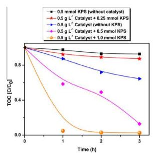
Fig. 9. Effect of potassium persulfate (KPS) [Experimental conditions: LaFeO<sub>3</sub> (0.5 g L<sup>-1</sup>), 4-chlorophenol ( $1.25 \times 10^{-4}$  M) and KPS were ultrasonicated (40 kHz) for 3 h].
