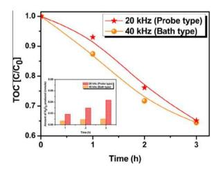
**Fig. 8.** Effect of ultrasound frequency [Experimental conditions: LaFeO<sub>3</sub> (0.5 g L<sup>-1</sup>) and 4-chlorophenol ( $1.25 \times 10^{-4}$  M) were ultrasonicated (20 kHz or 40 kHz) for 3 h] [inset: amount of H<sub>2</sub>O<sub>2</sub> (mmol) produced from each sonicator].
