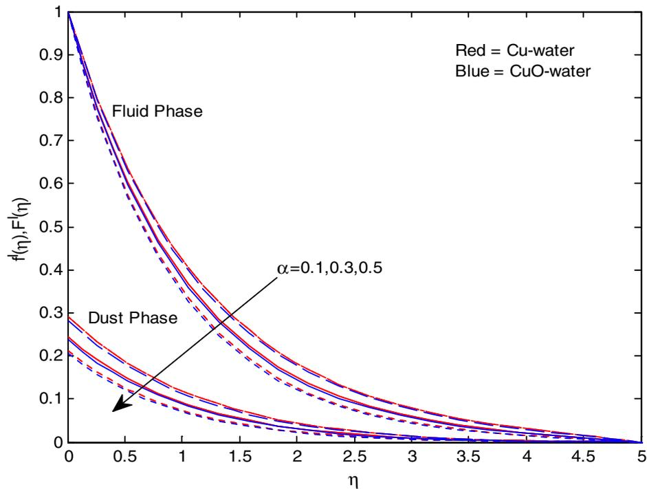
Fig. 9. Variation in velocity profiles of fluid and dust phases for different values of  $\alpha$ .
