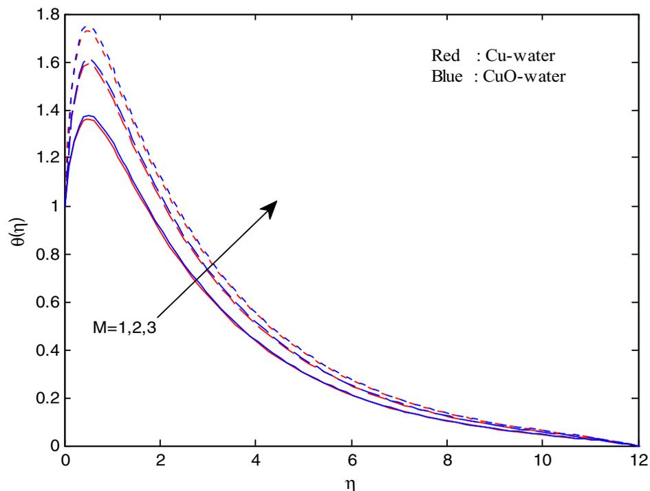
Fig. 12. Variation in temperature profiles for different values of  $M$ .
