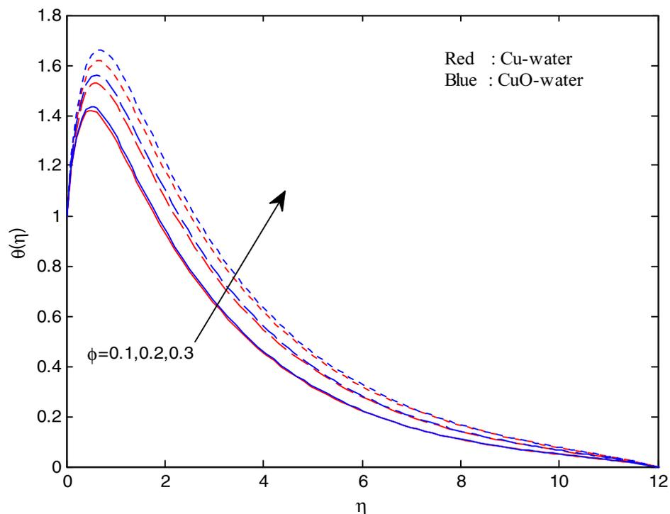
Fig. 4. Variation in temperature profiles for different values of  $\phi$ .
