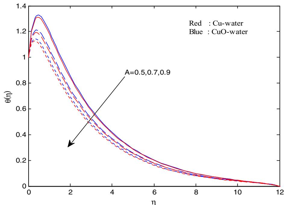
Fig. 6. Variation in temperature profiles for different values of  $A$ .
