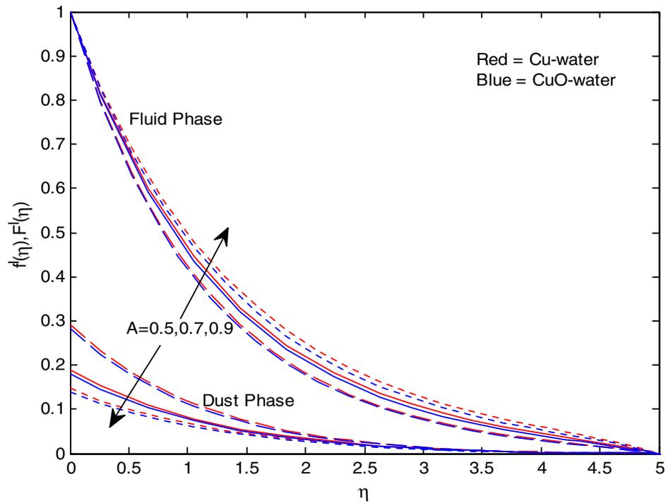
Fig. 5. Variation in velocity profiles of fluid and dust phases for different values of  $A$ .
