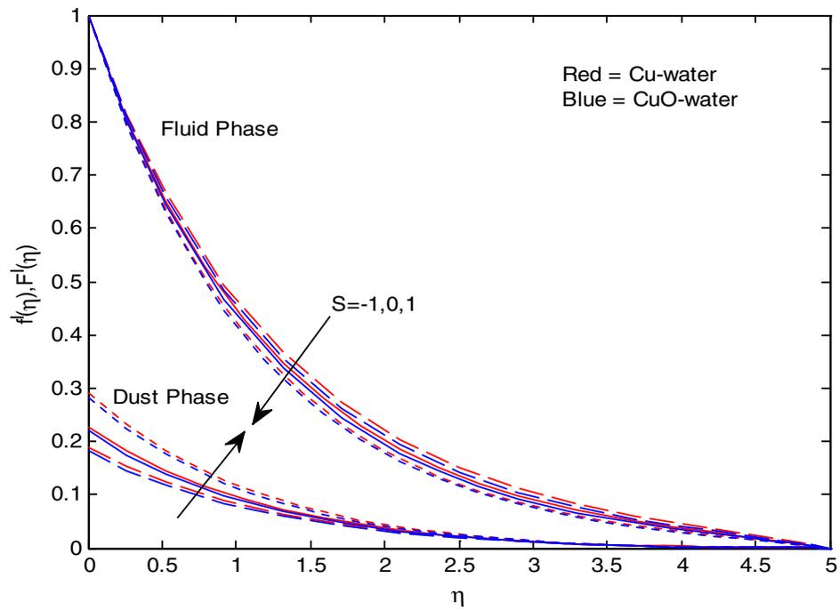
Fig. 16. Variation in velocity profiles of fluid and dust phases for different values of  $S$ .
