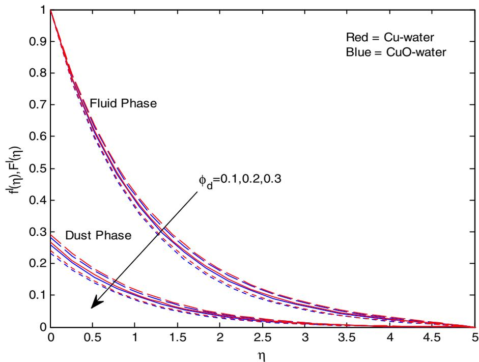
Fig. 1. Variation in velocity profiles of fluid and dust phases for different values of  $\phi_d$ .
