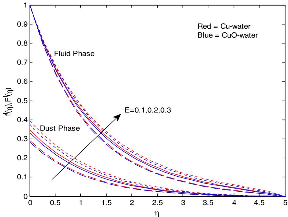
**Fig. 14.** Variation in velocity profiles of fluid and dust phases for different values of  $E$ .
