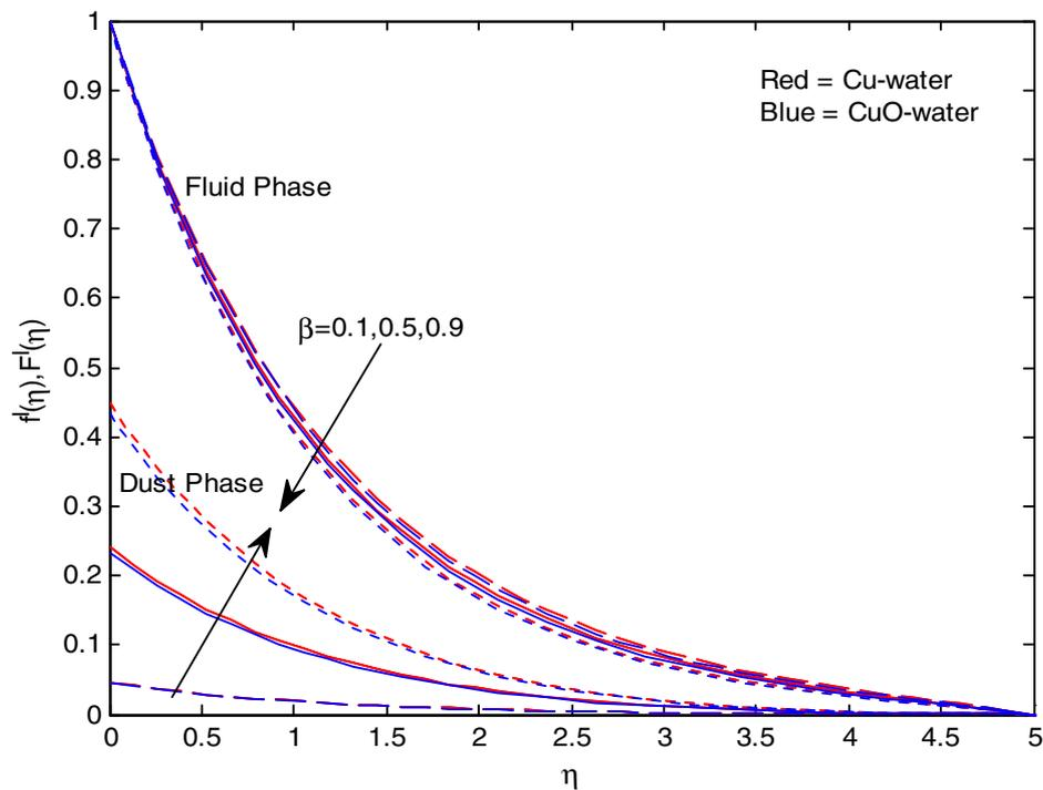
Fig. 7. Variation in velocity profiles of fluid and dust phases for different values of  $\beta$ .
