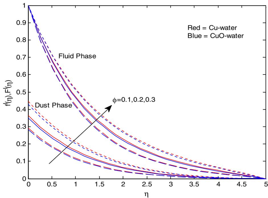
Fig. 3. Variation in velocity profiles of fluid and dust phases for different values of  $\phi$ .
