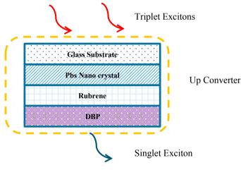
Fig. 5 Architecture of Up Converter
