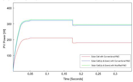
Fig. 7 (b) Comparison between Conventional & Modified P&O MPPT
