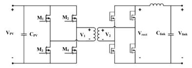
Fig. 7 (a) DC - DC Full Bridge Power Converter Circuit.
