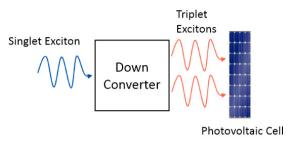
Fig. 2 Basic Scheme for down conversion.
