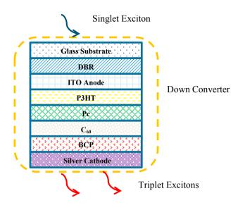
Fig. 3 Architecture of Down Converter
