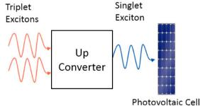
Fig. 4 Basic scheme for Up conversion.
