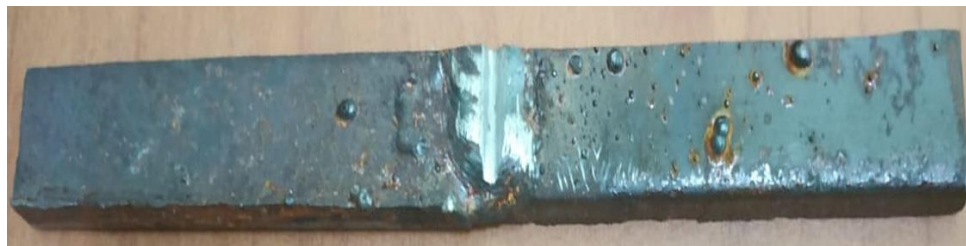
Figure 2. V-nose on the welded mild steel plate for impact test
