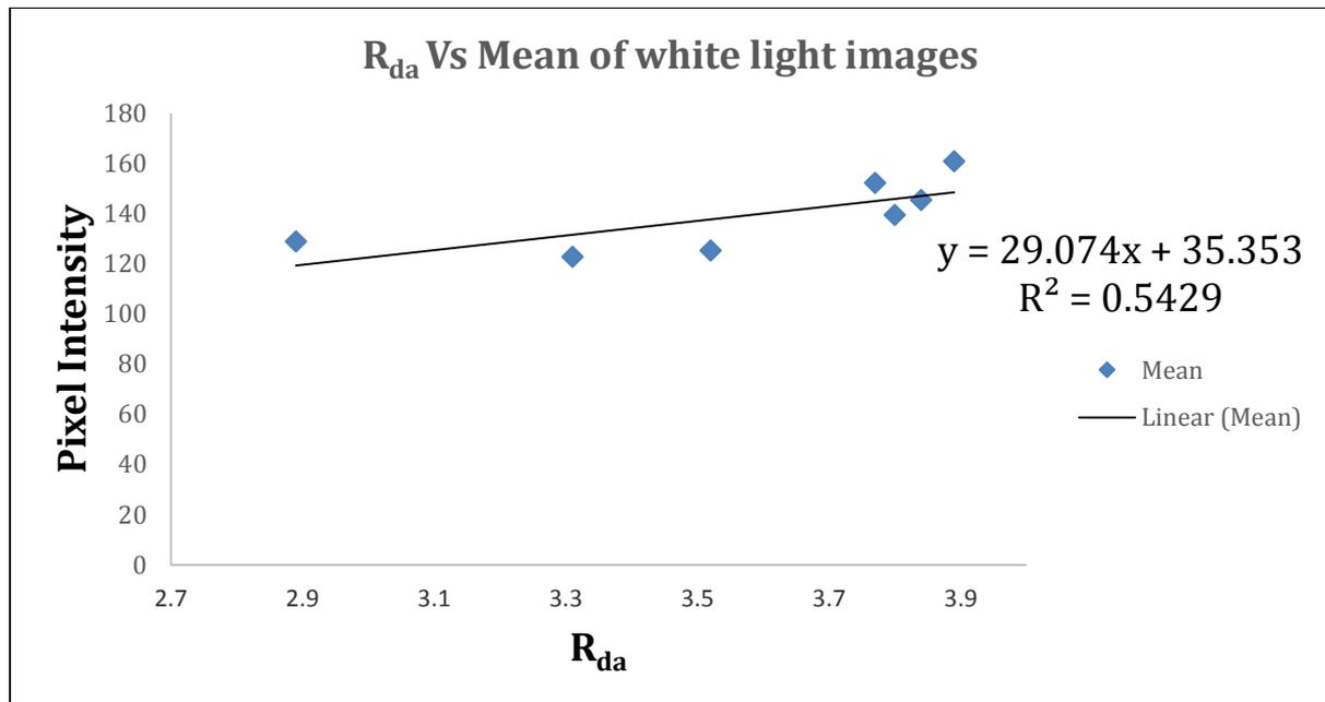
**Figure 11.** The correlation of mean of image intensity with R<sub>da</sub> for white light images.
