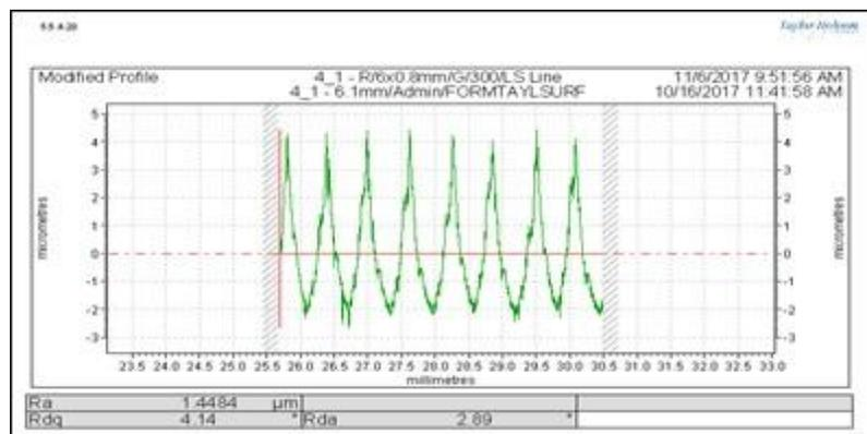
**Figure 4.** A Representative Surface roughness profile.
