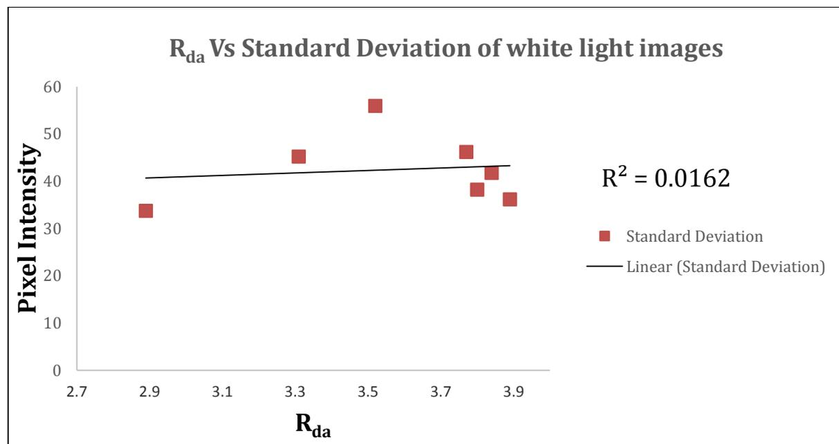
**Figure 12.** The correlation of standard deviation of image intensity with R<sub>da</sub> for white light images.
