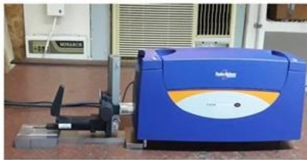
**Figure 3.** The Taylor and Hobson surface roughness tester (Talysurf).
