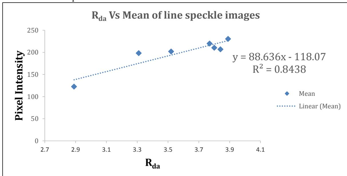
**Figure 9.** The correlation of mean of image intensity with  $R_{da}$  for line speckle images.
