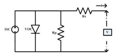
Fig. 3. Equivalent circuit of solar PV panel.
