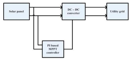
Fig. 2. Overall solar PV panel configuration.
