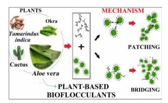
Figure 2 | Mechanism of flocculation using plant-based bioflocculants.
