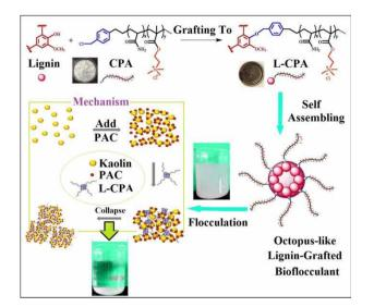
Figure 3 | Formulation of octopus-like lignin-grafted bioflocculant and its mechanism.
