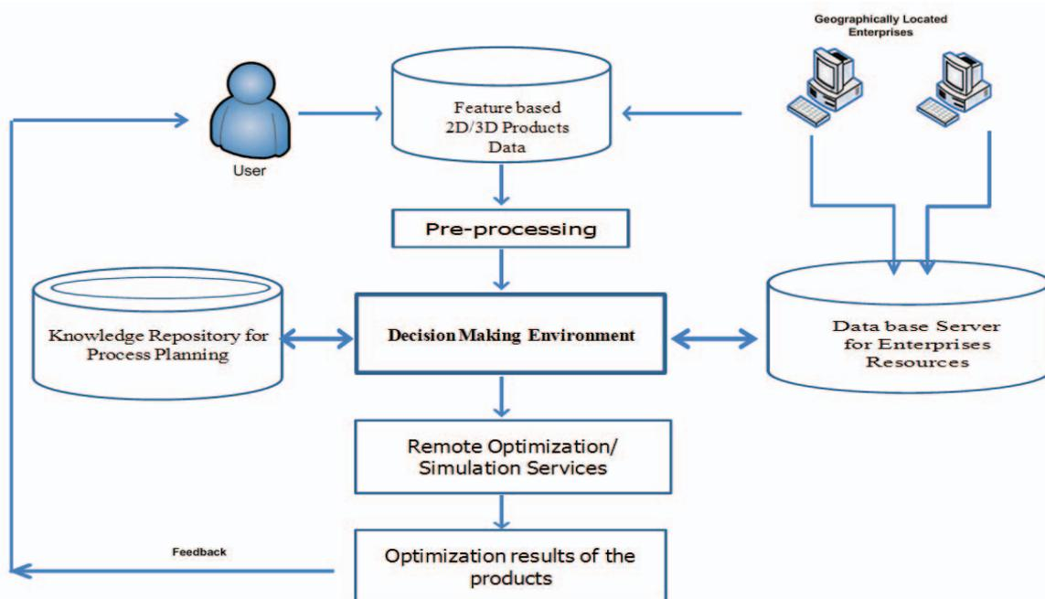
Figure 3 Web enabled system architecture.
