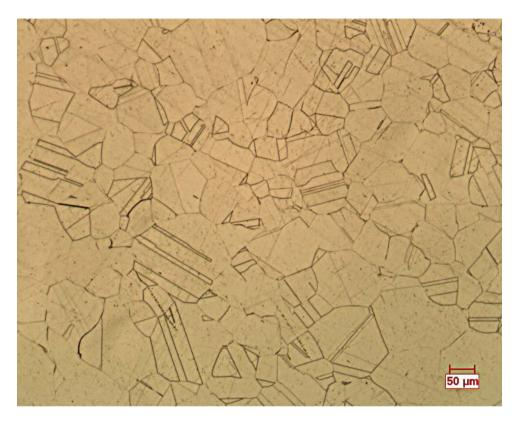
Figure 1. Microstructure of Hastelloy C-276 in as-received condition.
