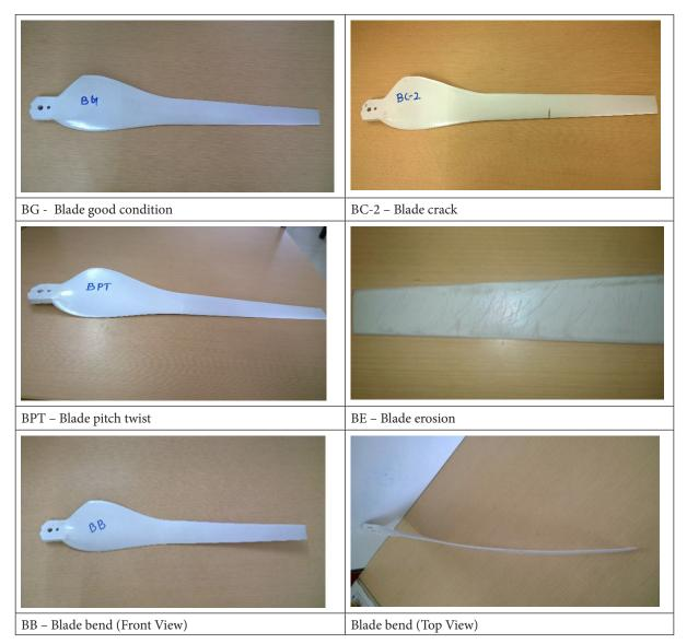
Figure 3. Different blade fault conditions (Considered)
